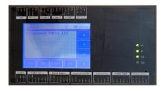
This enables integration with building management systems (BMS) and allows them to write measurement inputs to the PA Pro III and read back calculated results such as COP and System Efficiency Index.
